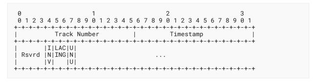
Figure 12: Block Header with 2 Octets TrackNumber
