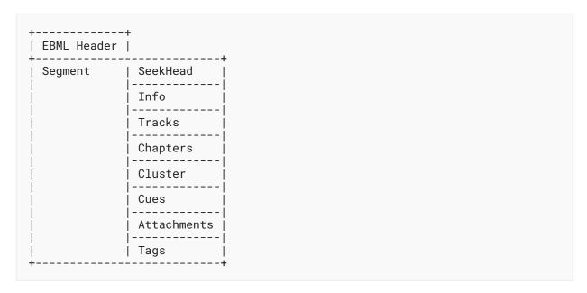
Figure 1: Basic Layout of a Matroska File
