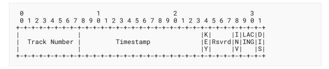
Figure 13: SimpleBlock Header with 1 Octet TrackNumber
