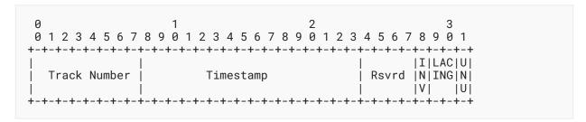
Figure 11: Block Header with 1 Octet TrackNumber
