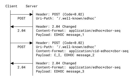
*Figure 11: Example of the Reverse Message Flow*
