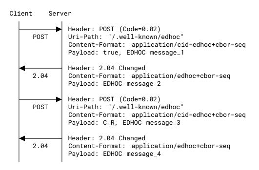
Figure 10: Example of the Forward Message Flow
