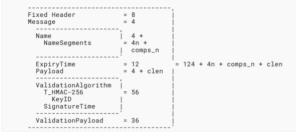
Figure 40: Estimated Size of an Uncompressed CCNx Content Object
