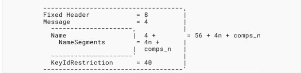
Figure 38: Estimated Size of an Uncompressed CCNx Interest
