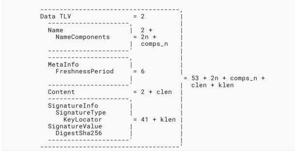
Figure 36: Estimated Size of an Uncompressed NDN Data
