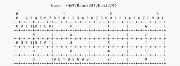
Figure 10: Name TLV Compression for /HAW/Room/481/Humid/99
