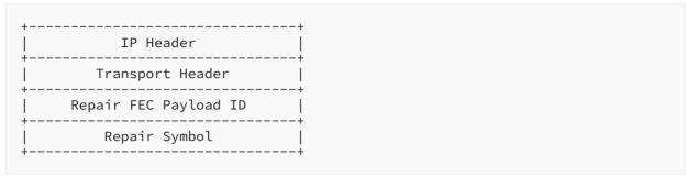
Figure 7: Structure of an FEC Repair Packet with the Repair FEC Payload ID
