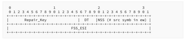
Figure 8: Repair FEC Payload ID Encoding Format
