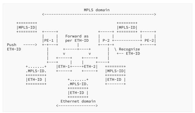
Figure 11: MPLS Nodes Interconnected by an Ethernet Domain
