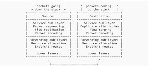
Figure 2: DetNet Data-Plane Protocol Stack
