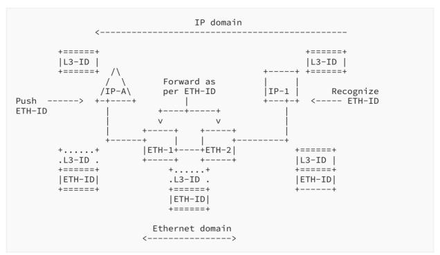
Figure 10: IP Nodes Interconnected by an Ethernet Domain
