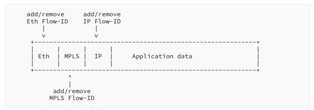
Figure 9: Packet with Multiple Flow-IDs
