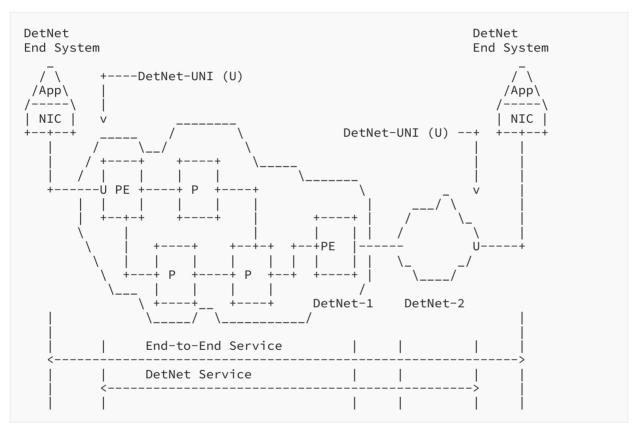
Figure 5: DetNet Service Reference Model (Multidomain)
