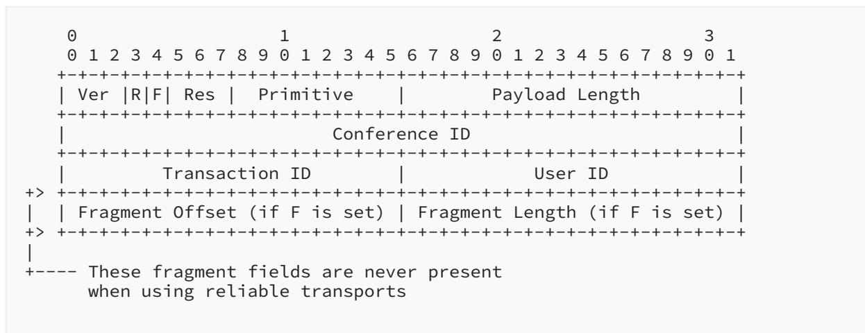
Figure 5: COMMON-HEADER format
