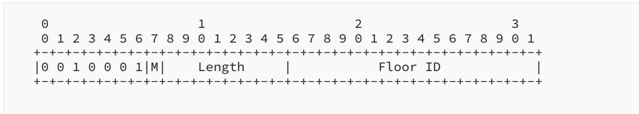
Figure 27: FLOOR-REQUEST-STATUS-HEADER format
