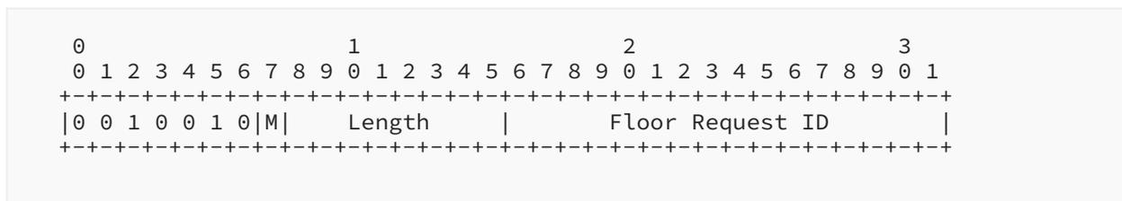
Figure 29: OVERALL-REQUEST-STATUS-HEADER format
