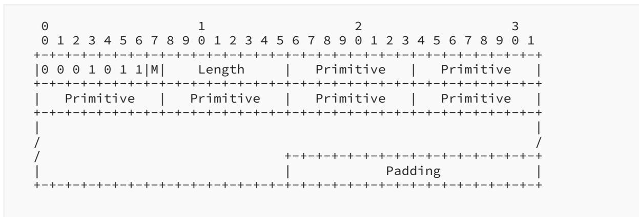
Figure 18: SUPPORTED-PRIMITIVES format
